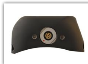
7-pin Fischer connection for three O 2 sensors and USB
